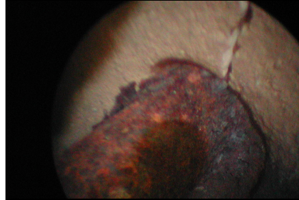
Corroded pin and cracked rib.
